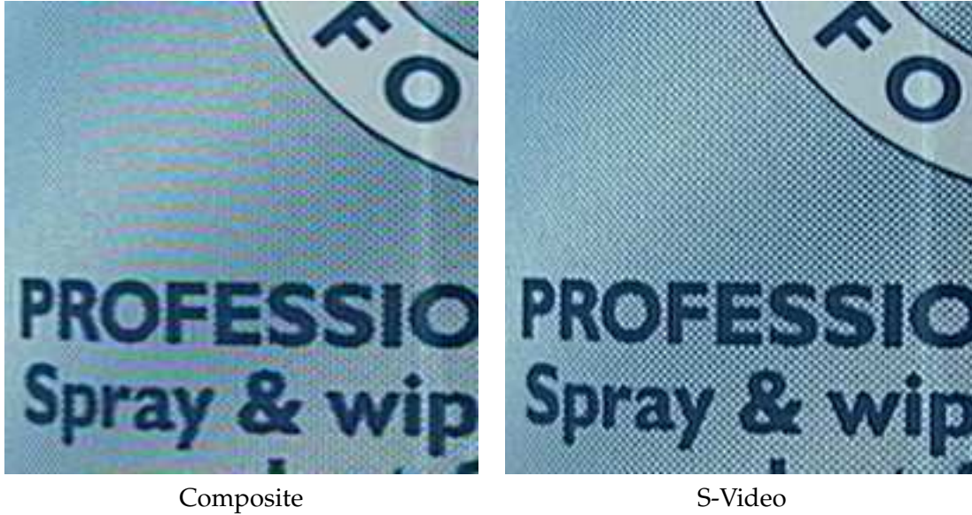
Figure 4.3: Comparison of S-Video and Composite Video
